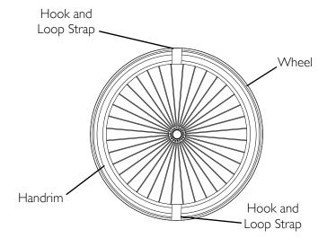
FIGURE 2 Removing/Installing Handrims with Tabs
